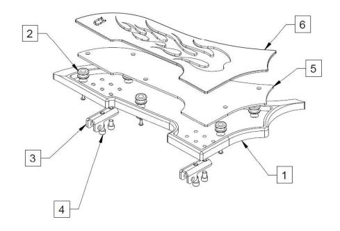
STEP 3. Assemble Lower Graphics Deck (5) with Top Deck (6) by aligning Upper Deck (6) stand-off through holes in Lower Deck (5).
