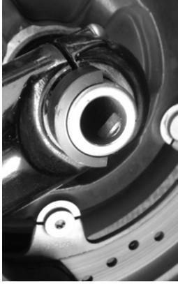
STEP 2. Using the Set Screws from the same bag as selected Spacer Sleeve, install Set Screws into an Axle Cover, but only thread partially into cover. **Before continuing, apply a small amount of Loctite onto each thread (this will prevent loosening due to vibration).**
