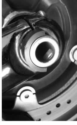
STEP 2. Using the Set Screws from the same bag as selected Spacer Sleeve, install Set Screws into an Axle Cover, but only thread partially into cover. **Before continuing, apply a small amount of Loctite onto each thread (this will prevent loosening due to vibration).**
