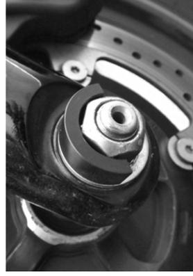
STEP 6. Using the Set Screws from the same bag as selected Spacer Sleeve, install Set Screws into an Axle Cover, but only thread partially into cover. **Before continuing, apply a small amount of Loctite onto each thread (this will prevent loosening due to vibration).**
