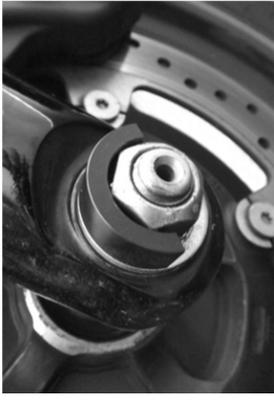
STEP 6. Using the Set Screws from the same bag as selected Spacer Sleeve, install Set Screws into an Axle Cover, but only thread partially into cover. **Before continuing, apply a small amount of Loctite onto each thread (this will prevent loosening due to vibration).**
